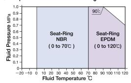
\*This table conforms to the JIS standard (JIS B 2032). Contact us if you operate your valve outside the above pressure and temperature ranges.
